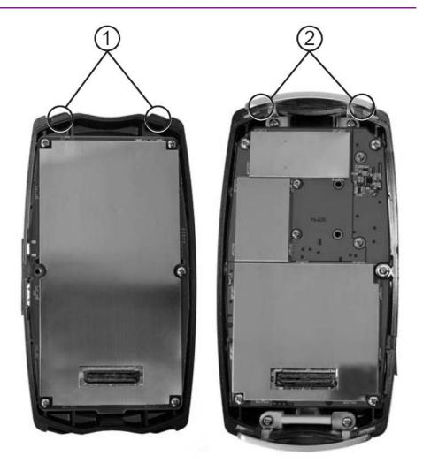
Figure 1.6-1 Alignment Tabs and Slots
