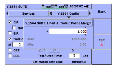
Figure 3.11.7-2 Y.1564 Config Setup – M Value Editor
